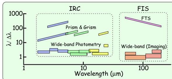
**Figure 1.** Wavelength coverage and spectral resolution of the IRC and FIS.
