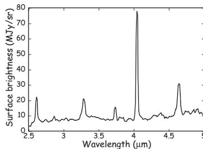
**Figure 5.** Example of the IRC NIR spectrum of a HII region taken during the warm mission phase. Strong emission features are mostly hydrogen recombination lines. The 3.3  $\mu\text{m}$  UIR band is also clearly seen.
