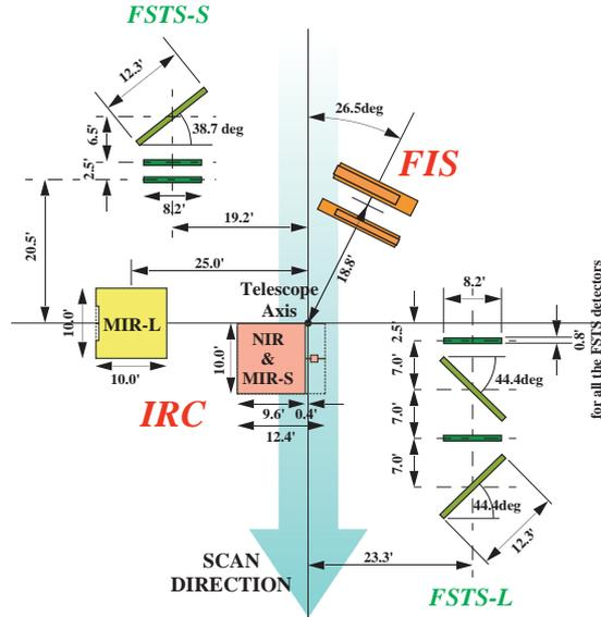
**Figure 2.** Focal-plane layout of *AKARI*. The scan direction in the all-sky survey is indicated by the large arrow. The field-of-view of WIDE-S and WIDE-L, and N60 and N160 overlap with each other as do NIR and MIR-S.
