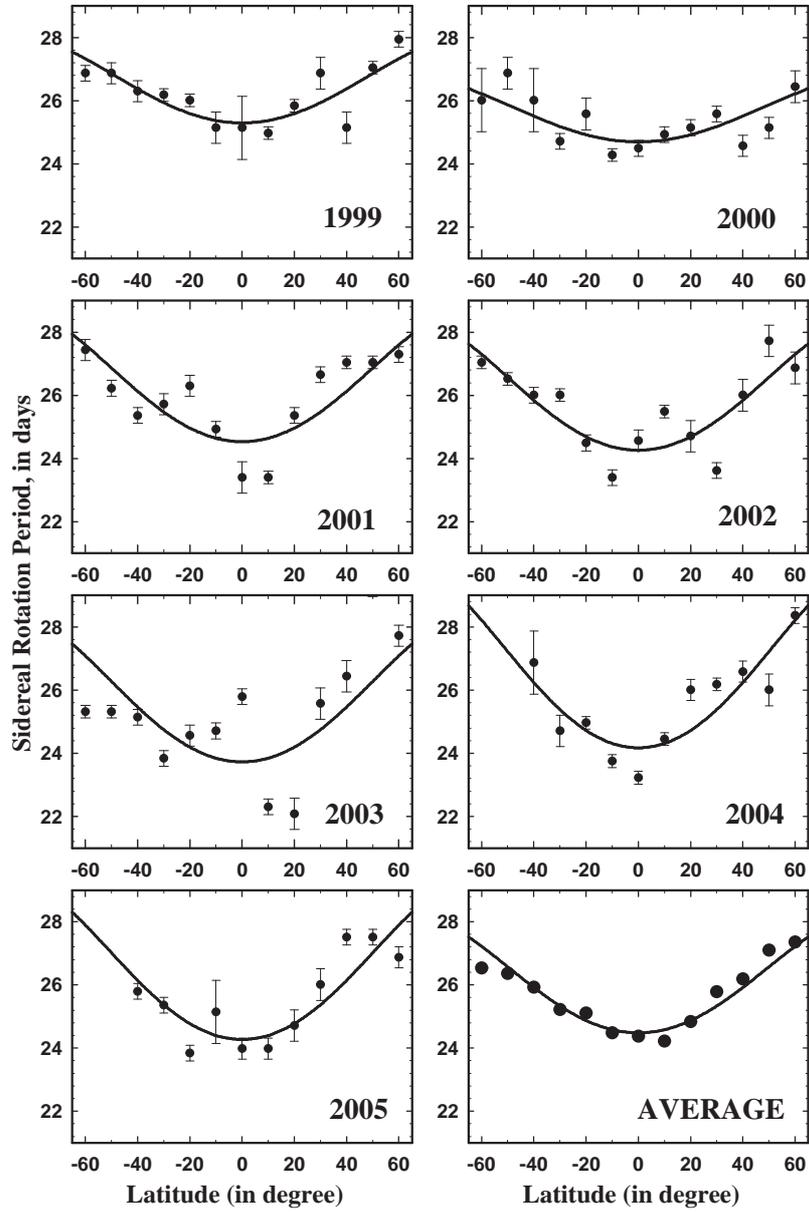
**Figure 1.** Sidereal rotation periods as a function of latitude. These are obtained from the radio images at 17 GHz of the years 1999-2005. The size of error bars depends on the selection of the peak in determination of the rotation period. The least square curves fitted in the rotation profiles of the sidereal period are also shown. The average rotation profile as a function of latitude is also plotted separately (last plate).
