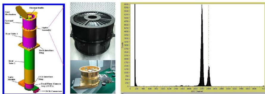
**Figure 5.** (i) A sketch of the SXT telescope, (ii) conical foil mirror assembly (above) and CCD housing (below), (iii) observed energy resolution for Fe55 radioactive source for an isolated pixel using engineering model.
