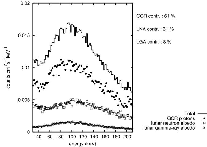
**Figure 1.** The total CZT background is represented by the solid line, the closed circles represent the contribution due to GCR protons, the open squares represent the contribution due to LNA, and the asterisks represent the contribution due to the LGRA.
