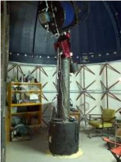
**Figure 2.** The stellar observatory: AstroSib 500 telescope mounted on a Paramount ME.
