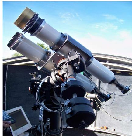
**Figure 3.** The solar observatory: suit of telescopes mounted on a Celestron CGEpro.
