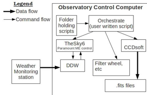
**Figure 1.** Data and command flow
