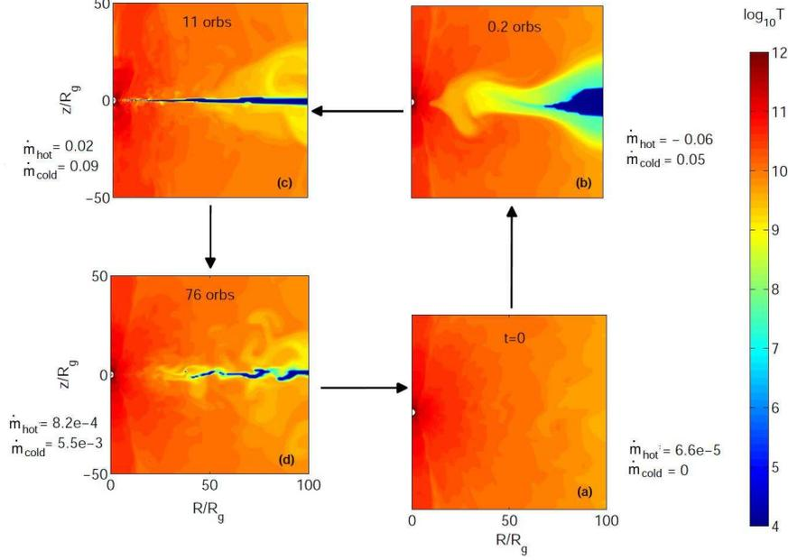
**Figure 1.** Complete state transition diagram from our idealized simulations. (a) Low-hard state (b) Intermediate hard state (c) High-soft state (d) Intermediate soft state.  $\dot{m}_{\text{hot}}$  and  $\dot{m}_{\text{cold}}$  are the accretion rates in units of  $\dot{M}_{\text{Edd}}$  of the hot and cold gas respectively. The grid resolution is  $256^2$  and  $\alpha = 0.1$ .
