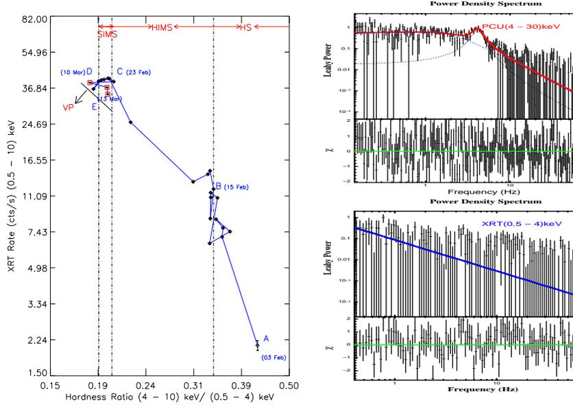
**Figure 2.** In Hardness Intensity Diagram (left), the states are demarcated by the vertical lines, except the Soft state (marked by red boxes) and the VP. Energy dependence of QPO (right) – the QPO is visible in the (4 – 30) keV range and is not seen in the soft photons (0.5 – 4) keV, which mostly arise from the Keplerian accretion disk. Power spectra are from 23 Feb (PCU) and 24 Feb (XRT) observations.
