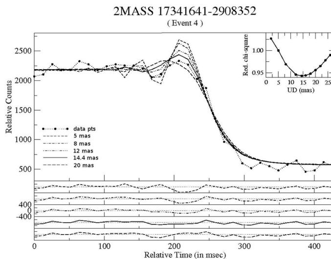
**Figure 2.** Galactic centre LO events: Event 4 data and model fits with various UD angular sizes. Best fit is at UD of 14.4 milli-arcsec as shown by minimum of inset error plot. Residuals (Data-Model) are shown at the bottom for angular sizes from 5 to 20 milliarcsec.
