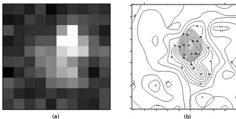
**Figure 1.** A sky subtracted subframe image and its contour plot. Each side of  $10 \times 10$  pixel sub-array is 5 arcsec. The seeing limited star image occupies  $3 \times 2$  arcsec in the subarray.
