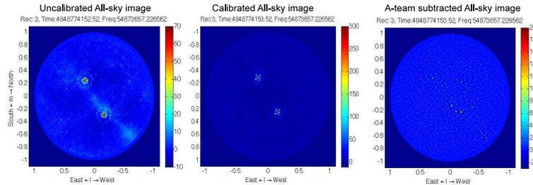
**Figure 1.** (left) An uncalibrated, instantaneous all sky image generated by the AARTFAAC (middle) the same timeslice after calibration (right) image after subtraction of the brightest sources reveals several bright 3C sources.
